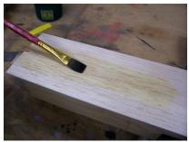
6. To mold the A-grain LE planking to the proper shape, first wet
