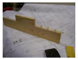
1. Make a jig from a board or strip of plywood <sup>3</sup>/<sub>4</sub>"X 3.5"
