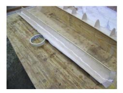
8. I covered the inside of the formed LE mold with epoxy finishing resin and .75 ounce fiber glass cloth by brushing the wet finishing resin on the wood, then dry brush the fiberglass on. I then coat the riblets and the outside edge of the 1/8" spar with the wet epoxy and while everything is still wet and uncured, I wrap the elastic bandage over it all to hold it in position. Be careful not to wrap too tightly as that can cause sagging between the riblets.
