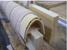
7. Once the balsa safely bends around the riblets, secure with two strips of masking tape and then wrap lightly with an elastic athletic wrap to hold in position. I sometimes do two at a time as shown in the photo, but one at a time works best. Let dry about 24 hours before removing.
