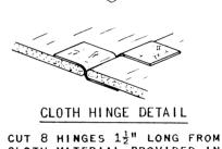
CLOTH MATERIAL PROVIDED IN KIT. CEMENT IN POSITION AS SHOWN ON STABILIZER SKETCH
